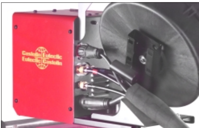
Fig.7g Interconnecting cable on the wirefeeder
